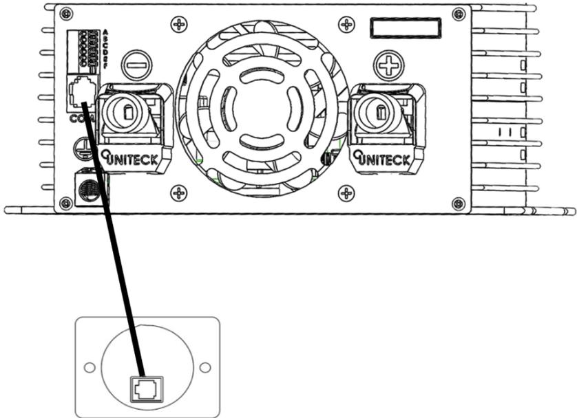
Once the connection has been made, put the switch on "remote" to enable the remote mode.
