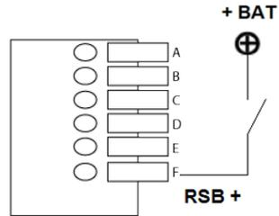
Once the connection has been made, put the switch on "remote" to enable the remote mode.
