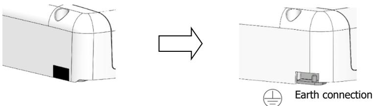
**Solar PV:** positive and negative pole of solar panels connection must not be connected at all to the earth. Connect only frame on your solar panels to earth to reduce lightning impact.
