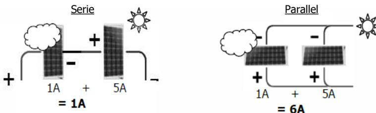
In case of parallel coupling, the panel current adds up.
