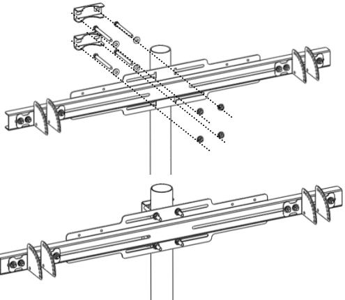
Unifix is equipped with a multi-position tilt system. (10 positions). Set the desired tilt depending on the desired orientation.
