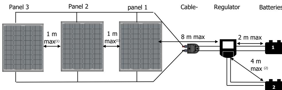
(1) Possibility to extend the distance between the panels by one additional meter, by adding a Unicable 612B and 612 R (cables not supplied with the Uniconnect 1.6 kit).
