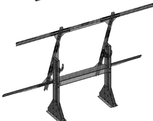
The angle of inclination can vary from 0 to 70 degrees.
